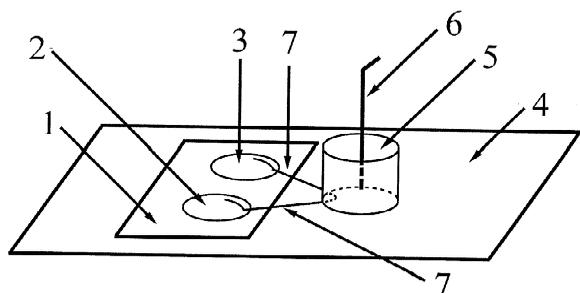
Fig. 1. Schematic diagram of the cell injector. (1) Transparency; (2) hole for the suspension of mast cell; (3) hole for the lysis solution; (4) microscope slide; (5) buffer reservoir; (6) anode for injection cell; (7) Ni wires.
